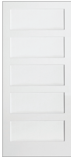
PR8755 1-3/8" (6/8) 3/8" MDF Flat Panel, Shaker Sticking
